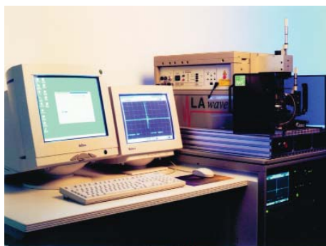
Fig. 2: Laser acoustic measuring device LAwave® for the non-destructive testing of thin films (Fig.: Fraunhofer IWS Dresden)
