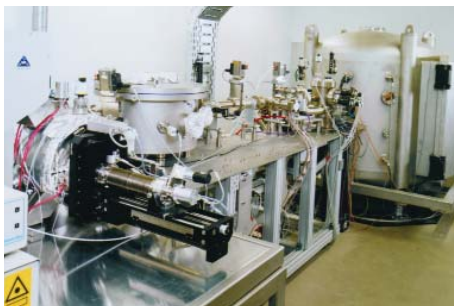
Fig. 1: Photograph of the laboratory EUV reflectometer (Fig.: Fraunhofer IWS Dresden)
