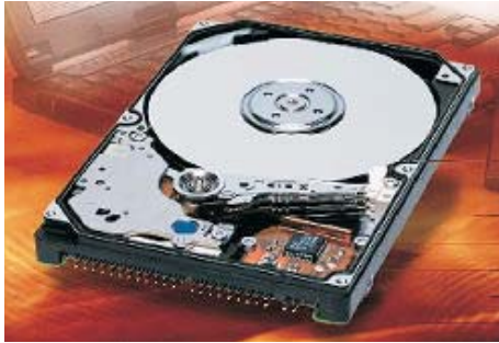
Fig. 1: IBM-microdrive, one of the smallest commercial drives presently available, capacity 1 GByte, weight 16 g, size 42.8 · 36.4 · 5 mm 3 , storage density 15.2 Gbit per square inch (Fig.: IBM Deutschland E&TS GmbH Mainz)
