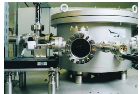
Fig. 3: Precision drive for the grating movements for the wavelength adjustment at the monochromator exit (Fig.: Fraunhofer IWS Dresden)
